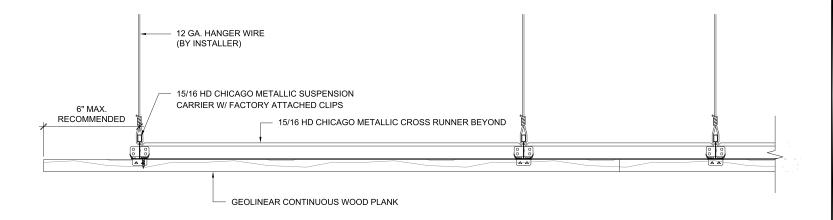
1/2" LONG SELF-TAPPING SCREW (BY INSTALLER) DRIVEN THROUGH GEOMETRIK SUSPENSION AT HOLE IN CLIP - EACH PLANK MUST BE SCREWED TO CLIP RAIL SYSTEM NEAREST THE JOINTS AND AT 4' O.C (MAX)
